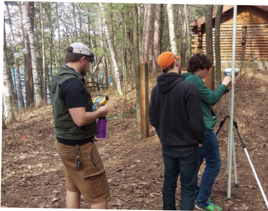
Students from Mobile GIS establish geographic positions using the TSC2 field computer and R6 GPS receiver.
