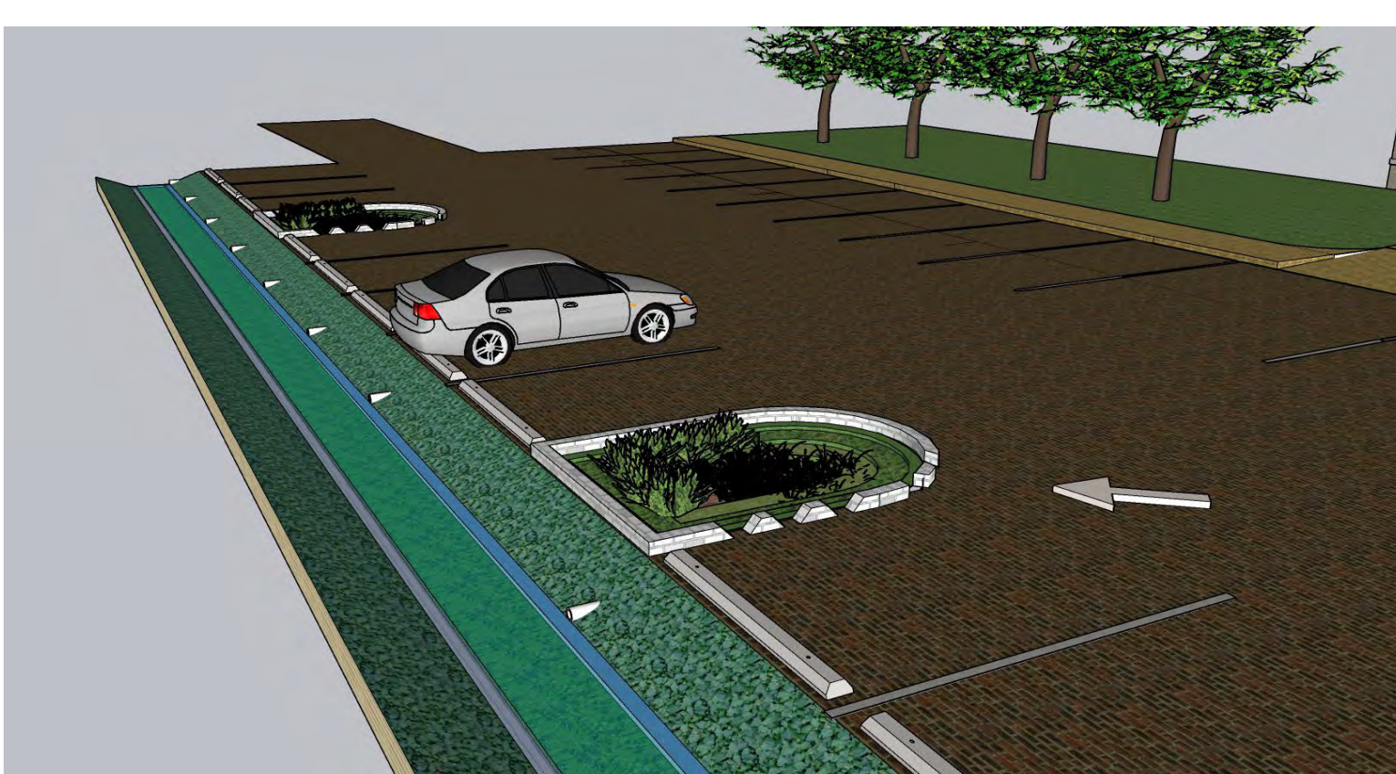
A bioswale parking lot that could be used to reduce and filter stormwater runoff.
