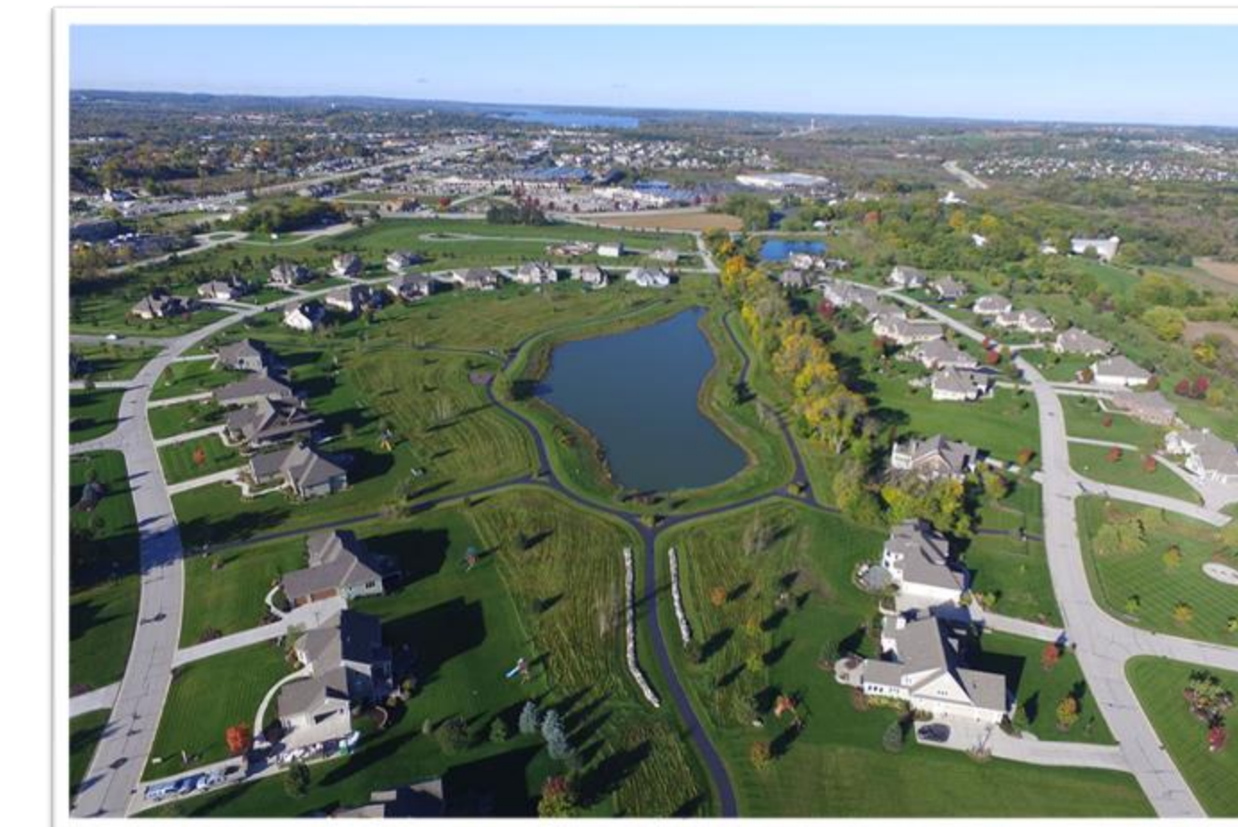
The aerial photo above shows the Hawksnest Conservation Subdivision in Delafield, Wisconsin. Note the ample open space, slightly smaller lot sizes, and trails characteristic of a conservation subdivision.
