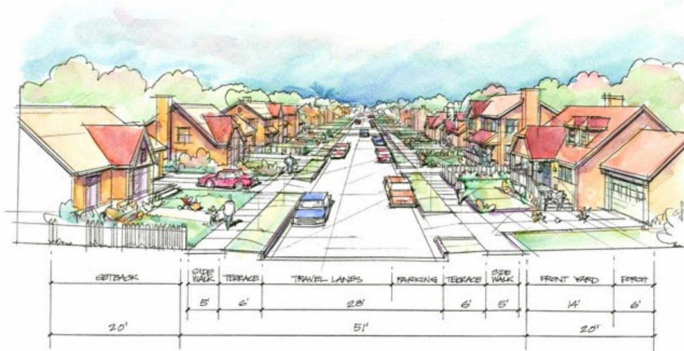
Example of a neighborhood street cross section: narrow streets and on-street parking help calm traffic and increase pedestrian safety
