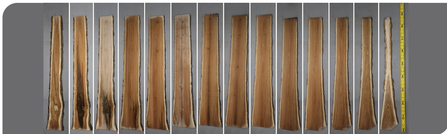
Figure 2. Boards were milled from Log F1, which was selected for a butt injury and a seam. Note the decay present in the first half of the boards.
