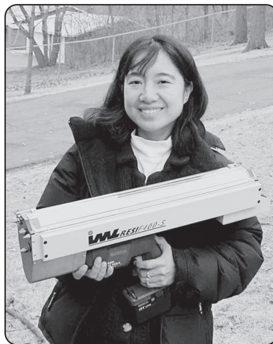
This machine helps Kyoko decide if a tree is hollow and should be cut down.
